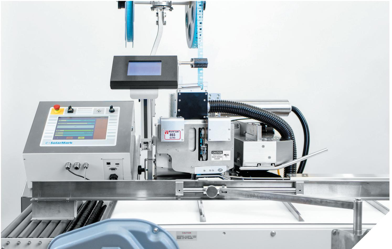
The eco-friendly, Kwik Lok 912 laser coding system is designed for maximum versatility. This fully automatic machine prints up to 120 closures per minute, is quick to install, and easy to use for over 100,000 working hours. Easily add permanent text, date, time, serial numbers, 2D codes and graphics onto your Kwik Lok closure while eliminating ink, solvents and waste.
