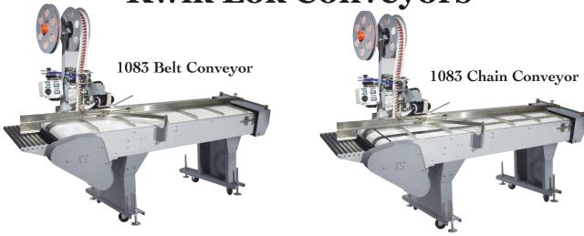
Kwik Lok conveyors can be order as a belt or chain version and will handle packages up to 20" (45 cm) in length at speeds of 60 or 90 packages per minute. Faster speeds, variable speed, and a kit to widen the conveyor are available. The conveyor can also be ordered with a brake-clutch unit that provides bag actuation. Conveyor lengths of 7.5' (2.29 m) to 30' (9.1 m) are available.
