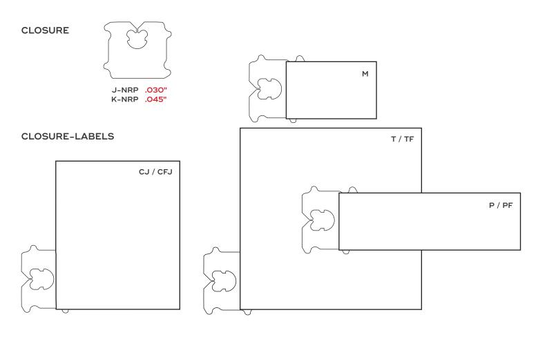
Various plastic thicknesses (in red) handle a wide range of package types, weights and sizes. Closures can be printed with price, date and/or code information.
