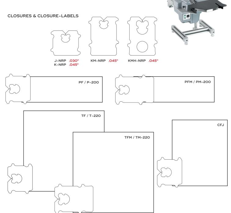
Various plastic thicknesses (in red) handle a wide range of package types, weights and sizes. Available colors vary with plastic thickness: .030'' - 7 colors .045'' - 3 colors
